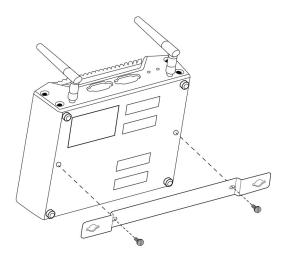
**Note:** The bracket must be oriented correctly to allow clearance for rubber pads on the bottom of the device.
