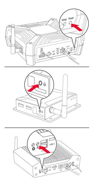
**Note:** The power button light comes on or starts blinking, and the indicator lights in the Ethernet port blink, go off, and then come on again.
